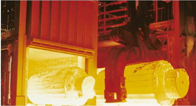
Metallurgical industry: forging furnace
