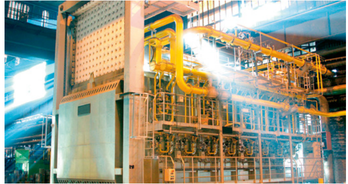
Ceramics industry: intermittent shuttle kiln
