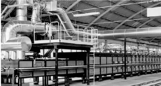
Roller hearth kiln in the ceramics industry
